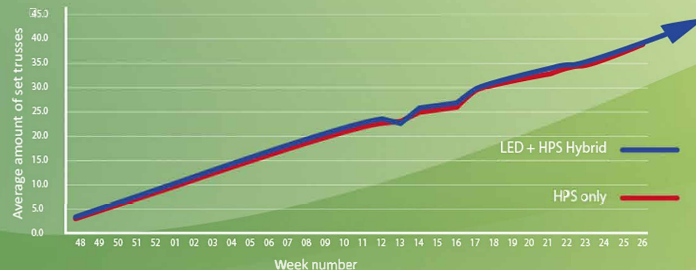
Graph 3: The average number of set tomato trusses was comparable under the two lighting setups, demonstrating that the LEDs did not affect pollination.
