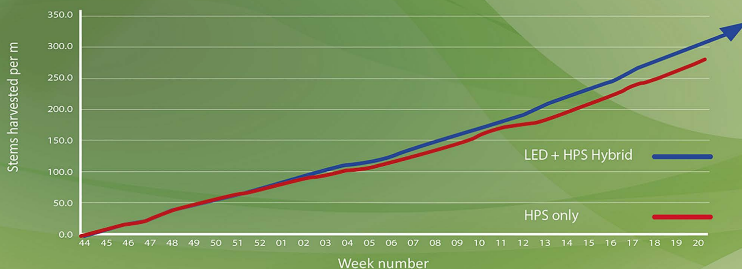
Graph 5: The cumulative number of gerbera daisy stems harvested per square metre. The hybrid LED+HPS setup saw 27.3 more stems harvested than under HPS-only lighting.
