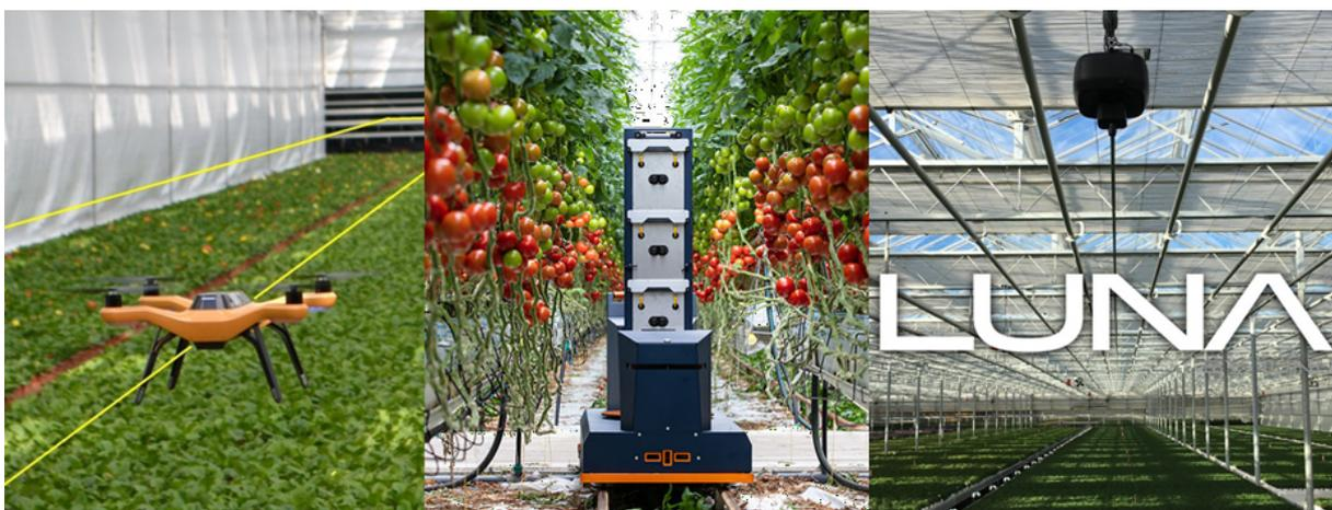
Figure 2 Corvus' autonomous drone, Hortikey's Plantalyzer and IUNU's LUNA
