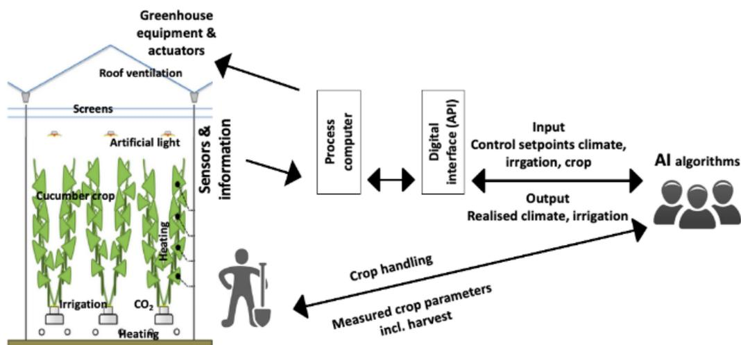
Figure 1 Scheme of data exchange in the first autonomous greenhouse challenge (Hemming et al., 2019)
