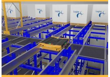
By using only 3D-Carrier's, that can move throughout the entire iCube and VT's (Vertical Transporters) movement between levels we managed to keep the logistical design of the iCube brilliantly simple. Since the 3D-Carrier and the VT's use only their own sensors, there's no need for other sensors in the iCube.
