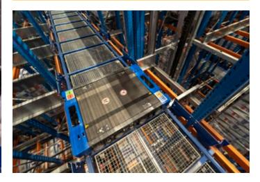
Depending on system size and throughput requirements the iCUBE can be equipped with as little as one 3D-Carrier and one Lift. If the size and/or throughput requirements of the warehouse are higher, the system can be equipped with as many 3D-Carriers and Lifts as needed. And since all machine movements are automatically controlled by our software, several 3D-Carriers can work together to complete high priority tasks quickly.
