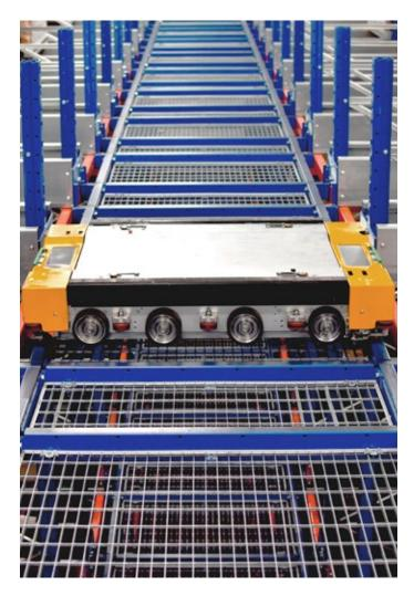
Safety zones can be configured in the iCUBE, so that the 3D-Carriers can keep executing tasks in the rest of the warehouse, while a certain zone of the warehouse becomes no-limit to the 3D-Carriers.
