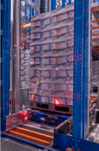
For warehouses where high availability is paramount, the system can also be equipped with more X-tracks (side movement tracks between aisles for the 3D-carriers) so that the 3D-Carriers can reach individual pallets even faster.
