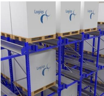
The iCUBE operates all the pallet movements using only the Logiqs 3D-Carriers and Vertical Transporters (VT).
