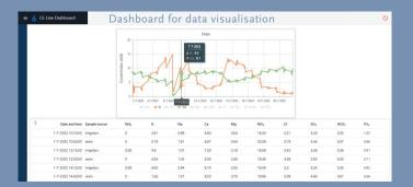
Selection of macronutrients and micronutrients: NH4, K, Na, Mg, Ca, Cl, NO3, SO4, HCO3, PO4 Fe, B, Zn, Mn, Mo, Cu
