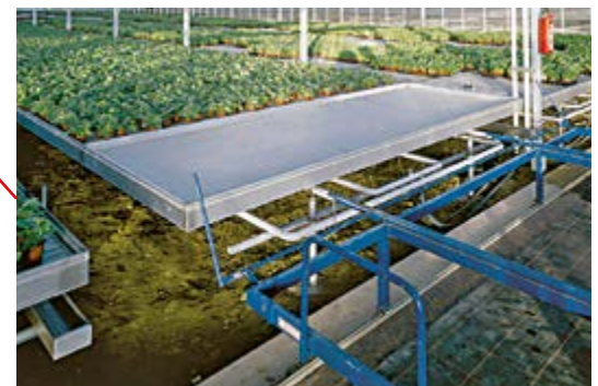
Track-guided, manual transport trolley with interlocking system
