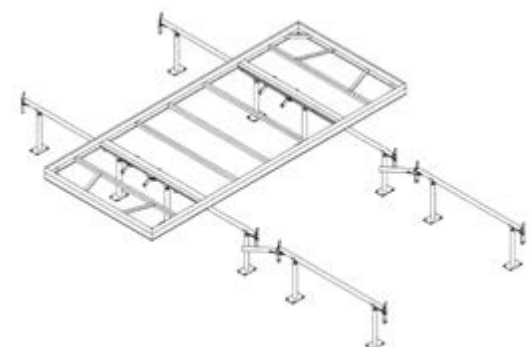
Rolling mobile bench onto a working position (hinged sections)
