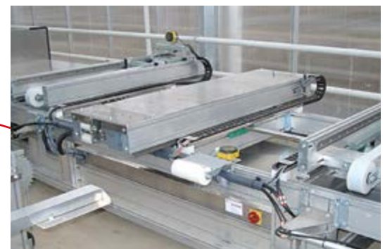
Automatic single or multi-layer transport robots for the loading and removal of benches
