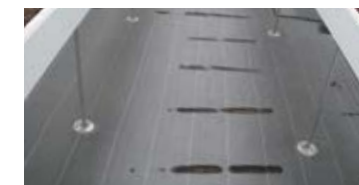
Burned holes in ground sheet
