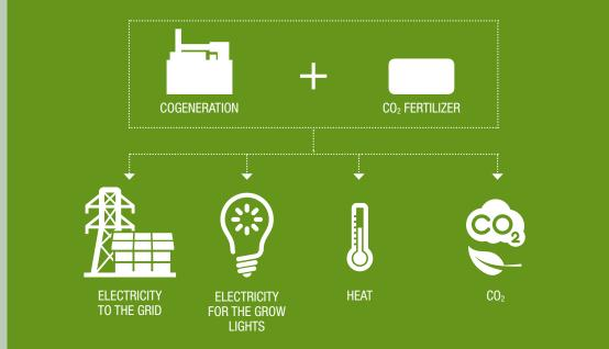
Cogeneration is based on the simultaneous production of electricity and recoverable heat, starting from a single source (both fossil and renewable), within a single integrated system. The main advantage compared to traditional separate-process energy production is that the heat is reused, while it normally remains unused and is released into the atmosphere.
