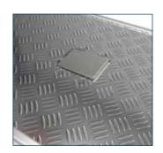
Because the foot pedal comes flush with the level of the platform, this increases the ergonomic posture for the employee
