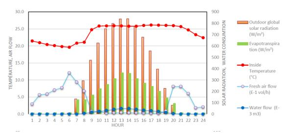
During night time and morning, external air is blow in the semi-closed greenhouse to dehumidify. During day time, pad is activated to cool.
