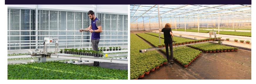
The SmartFlo Flexit provides flexible access to the SmartFlo Track. The SmartFlo Flexit consists of a belt with a mobile connection to the SmartFlo Track, giving easy access to the plants being transported, whether you want to set them down on, or pick them up from, the greenhouse floor. This can be communicated to the route concerned using an integrated SmartFlo Drive.
