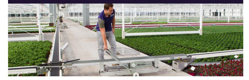
Another option to cross main aisles with the system, is by using a SmartFlo Crossover. To connect two opposite SmartFlo Tracks this unit can be inserted between both tracks to bridge the main aisle.
